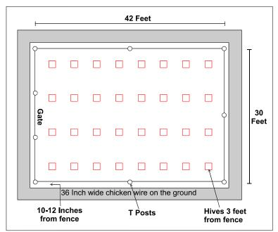
Figure 1. Top view of a temporary woven-wire electric fence and a temporary high-tensile electric fence designed to protect beehives from bears, showing spacing of posts and the position of beehives and chicken wire grounding apron relative to the woven-wire electric fence. Another "T" post is added to each of the longer sides of the temporary high-tensile electric fence.
