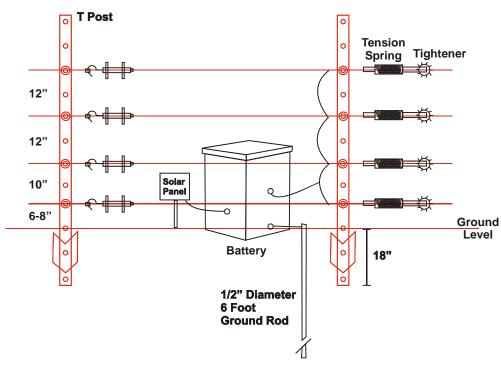
Figure 3. Side view of high tensile wire electric fence.
