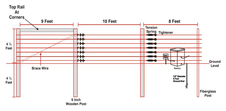
Figure 5. Side view of a permanent high-tensile electric wire fence.
