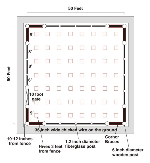
Figure 4. Top view of a permanent high-tensile electric wire fence designed to protect beehives from bears, showing spacing of posts and the position of beehives and chicken wire grounding apron relative to the fence.
