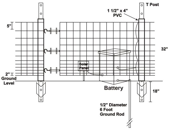
Figure 2. Side-view of a woven-wire electric fence is built with nine steel T-posts driven vertically into the ground.
